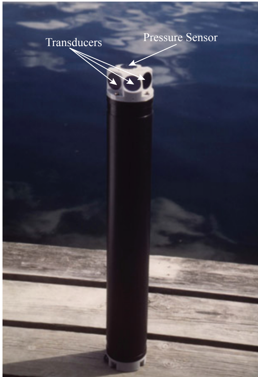
Figure 19. A photograph of an Aquadopp Acoustic Profiler (AP) manufactured by Nortek-AS. The AP emits pulses of energy that are reflected from scatterers carried by the water. The return pulse has a change in frequency called a Doppler shift. Because Doppler shift is proportional to the component of water flow along the beam, trigonometry is used to convert the returned acoustic signal into eastward, northward, and vertical components of water flow. This photo is courtesy of Nortek.
