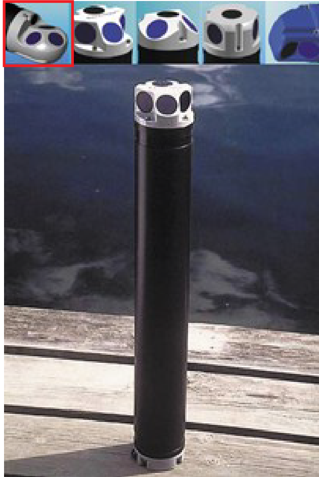
Figure 19a. A photograph of sensor head configurations that are available for the Nortek Aquadopp AP. The Aquadopp deployed in this study was configured with the right-angle sensor head (outlined in red on the photo), which is optimized for a low profile to minimize drag. This photo is courtesy of Nortek.
