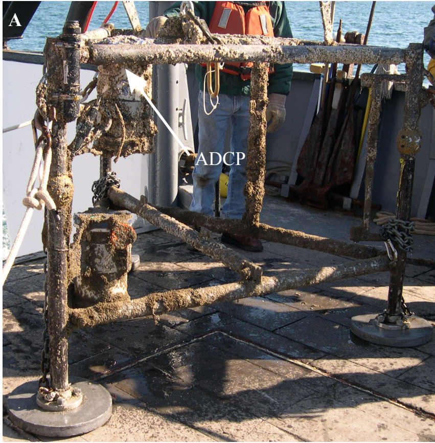
Figure 30. (A) A photograph of the tripod recovered from Site 1 at the end of the first deployment. (B) A photograph of the ADCP mounted to the tripod shown in (A). The ADCP and tripod are both heavily biofouled.
