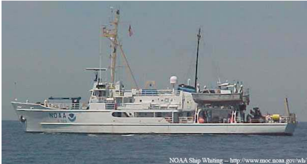
Figure 3.1. Photograph of the NOAA Ship Whiting. The Whiting, 163' long and equipped with two launches to carry out hydrographic surveys, was decommissioned by NOAA in 2003.
