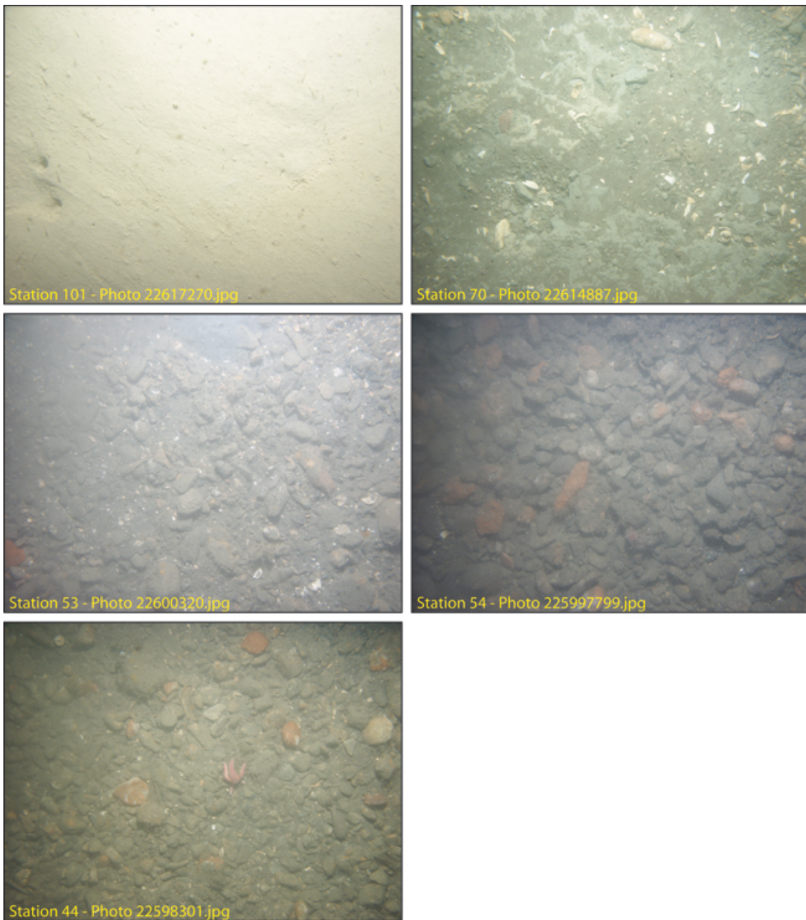
Figure 4.9. Photographs of the sea floor along the navigation channel, showing the transition for fine-grained mud in the inner harbor to a gravel pavement in the outer harbor (stations 101, 70, 53, 54, and 44). See figure 4.3 for station locations. See Appendix 3 for more photographs at these stations. The field of view of each image is approximately 50 cm wide.
