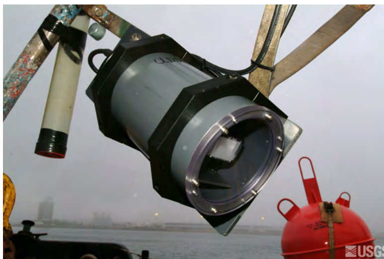
Figure 8. New bottom camera (top) and strobe (bottom) mounted on tripod prior to test deployment.
