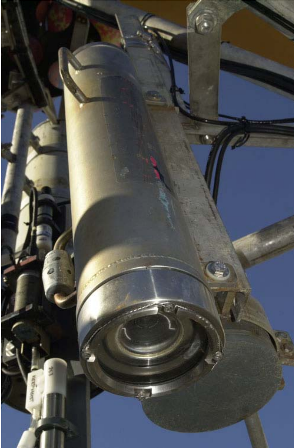
Figure 4. Benthos 35 mm underwater camera mounted on tripod frame. See figs. 2 and 3 for overview of frame.
