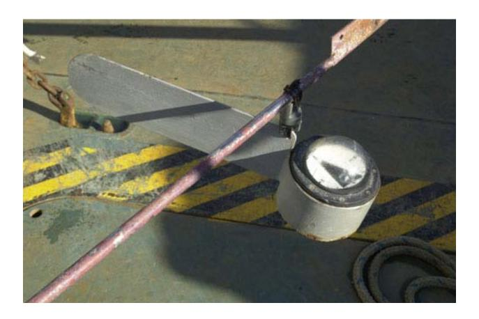
Figure 6. Compass and vane assembly mounted in the field of view of the camera. The vane orients in the current and shows the flow direction when the pictures are taken; the compass indicates magnetic north (16 degrees west of true north at LT-A).
